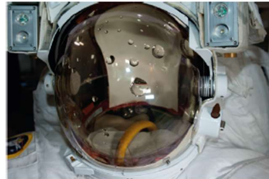
Figure 5. Extravehicular Mobility Unit (EMU) With Water in Helmet During Post-EVA 23 Screening Test
